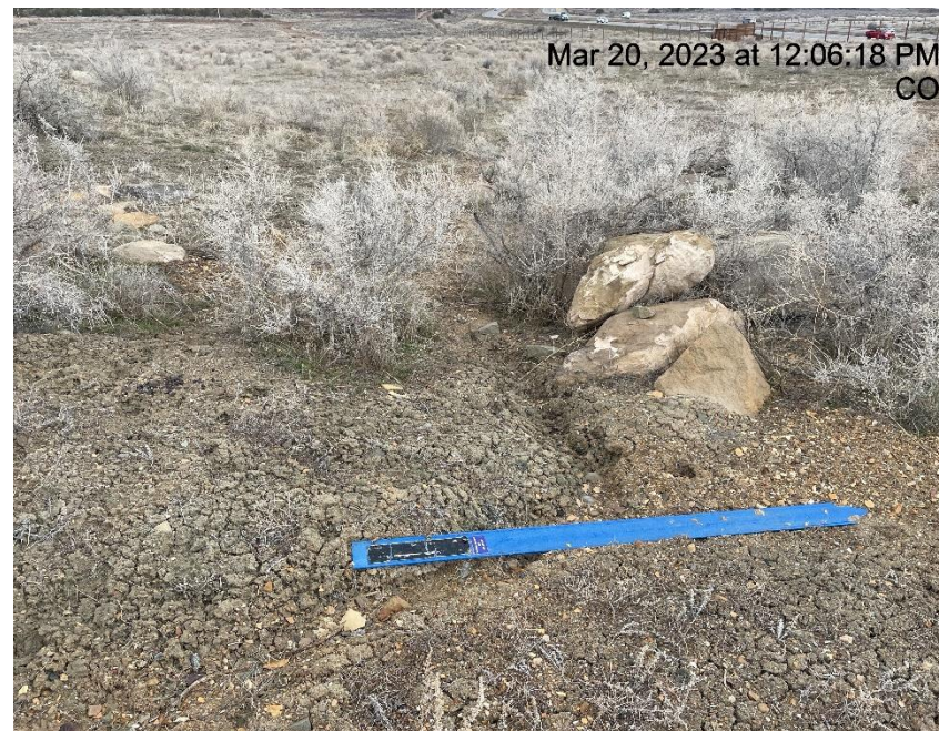
Photo # 2663 Rill erosion on spur road
