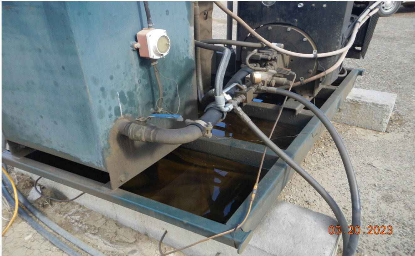
Photo 5. There is oil in the engine skid that needs to be cleaned up.
