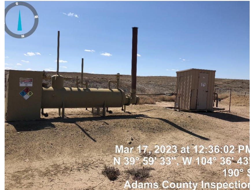
Photo#2 Separator/Gas Meter
