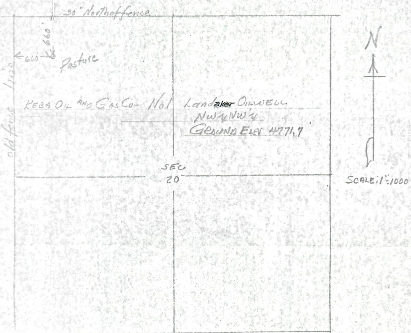
I hereby certify that the above plat is an accurate representation of a correct survey showing the location of Keba Oil and Gas Co.- No. 1 Landaker Oilwell in NW 1/4 NW 1/4 Sec. 20 T3S R55W 6PM. The elevation of the ground at the stake is 4771.7 feet above sea level from U.S.C.&G. Bench Mark.
