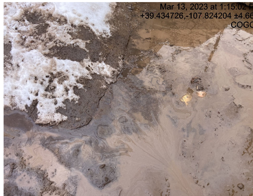
Staining and hydro carbon sheen on water
