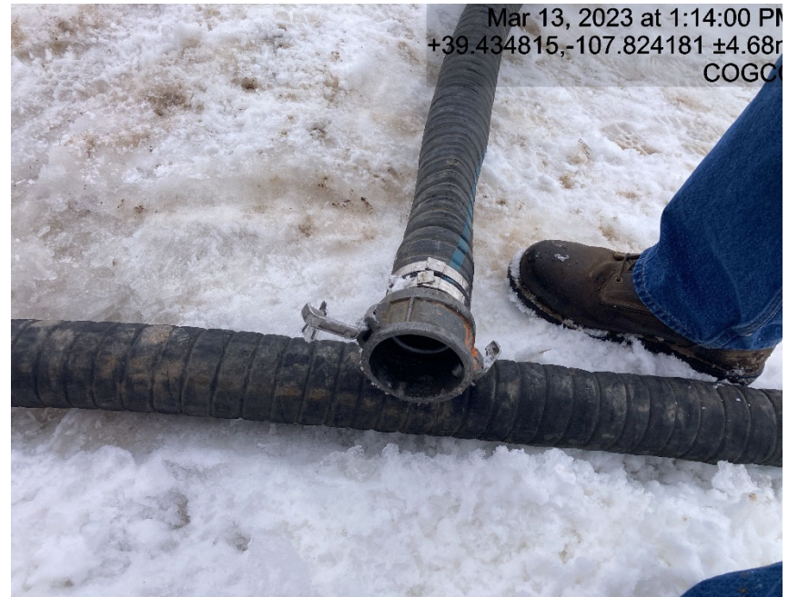
Hose hooked to frack tank missing cap
