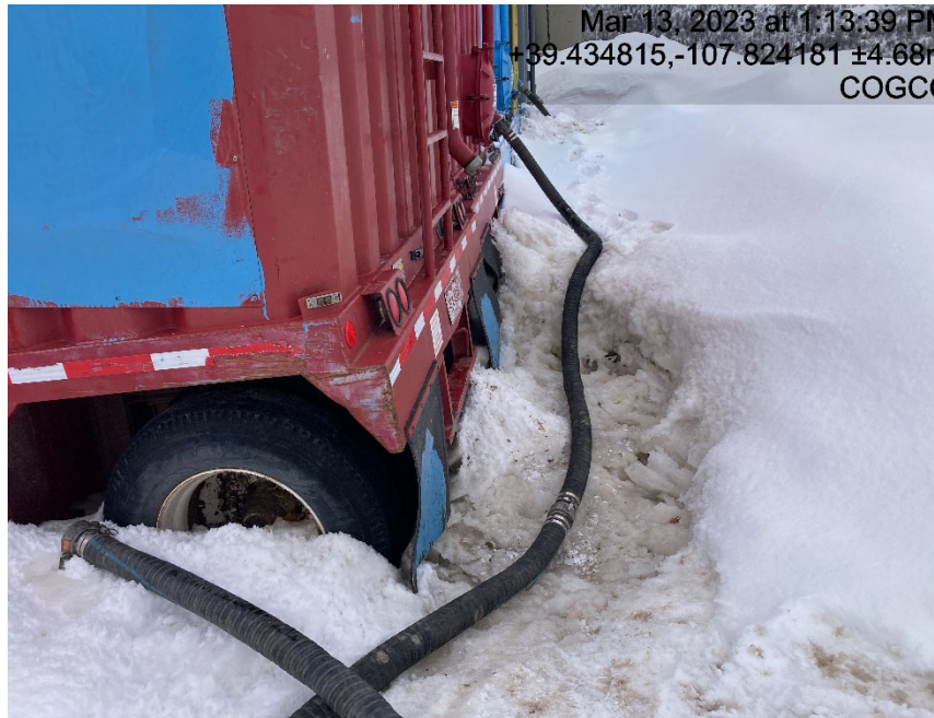
Hose hooked to frack tank missing cap
