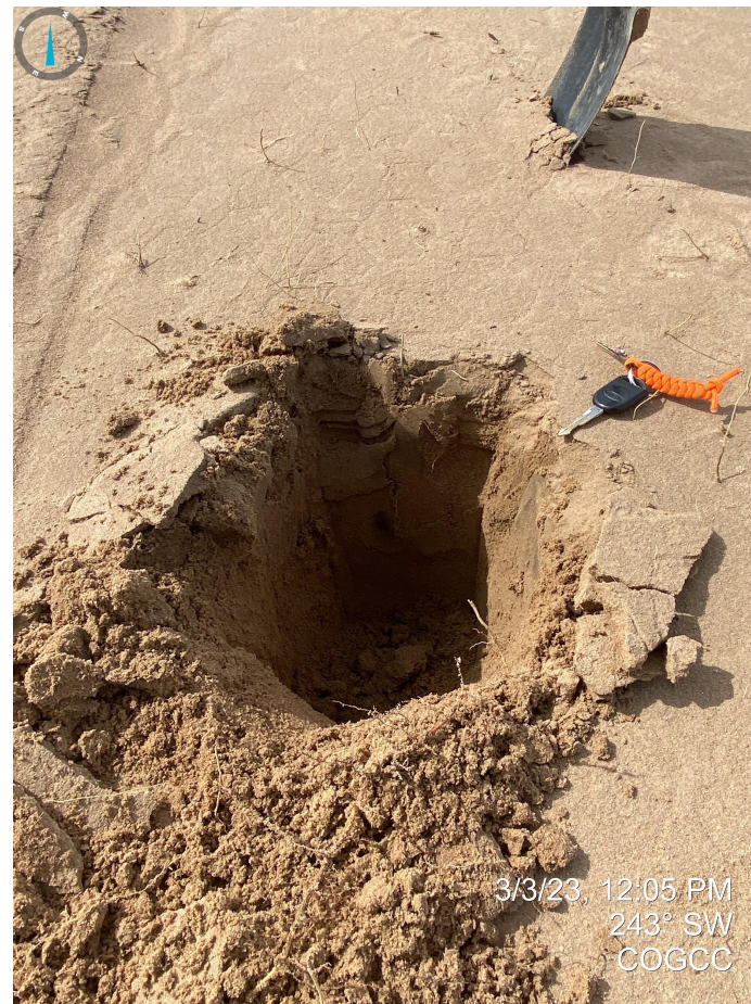
Photo 14. Facing southwest near the approximate center of the location. Soil pit dug by Staff to view soil profile; it appears the operator has salvaged all topsoil from the location.
