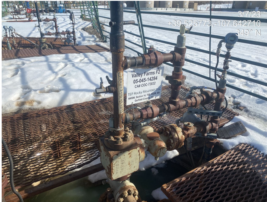
Photo 2. Photos show well API # 045-14284. Bubbles were rising in stormwater within the well cellar, indicative of a potential leak.
