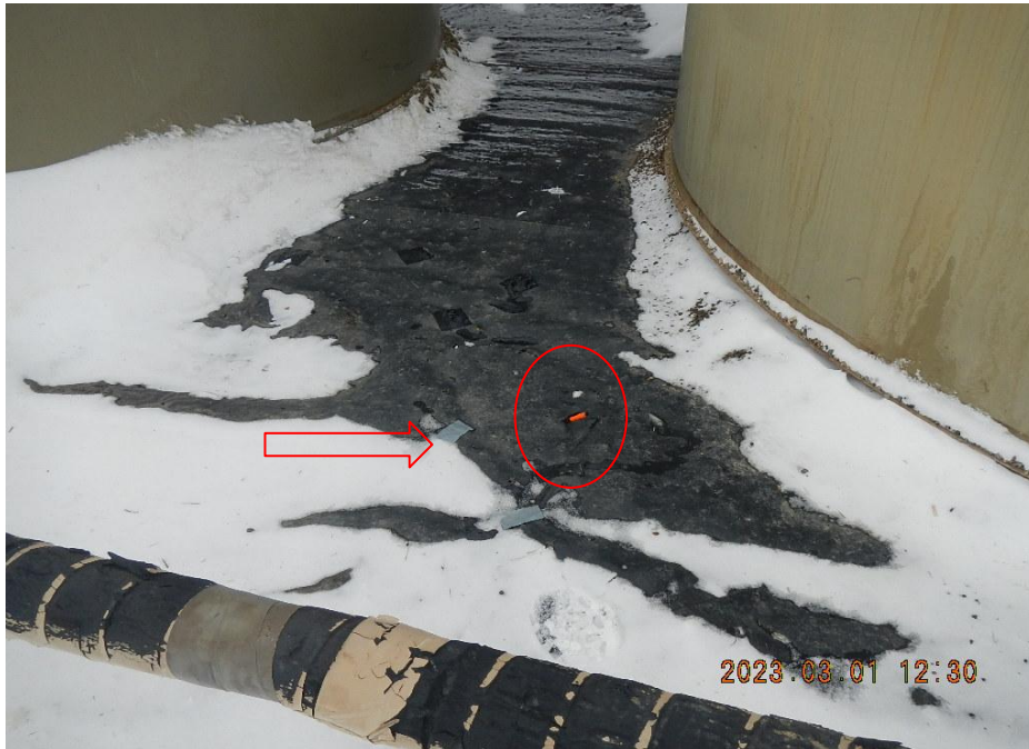
Photo 4. Liner with holes and repair. Note: Arrow points to Duct Tape repair. Circle depicts pen through liner penetration.
