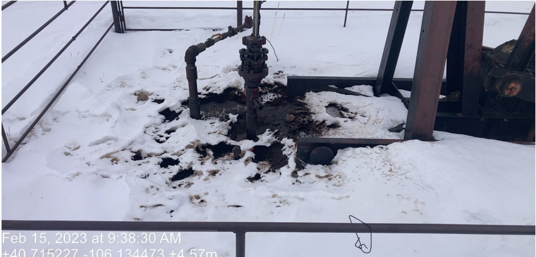
Previous inspection of staining and leaking stuffing box
