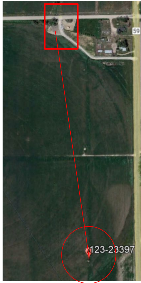
Photo 1. Google Earth aerial imagery taken 7/2019 during active operations. Photo illustrates the well location (red circle), tank battery (red rectangle), and approximate flowlines (red line).
