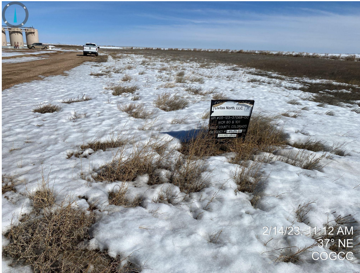
Photo 1. Facing northeast near the location's entrance. Photo illustrates that undesirable vegetation was observed throughout the interim reclamation areas. The operator will need to manage the location for undesirable vegetation during the next growing season to ensure compliance with Rule 1003.
