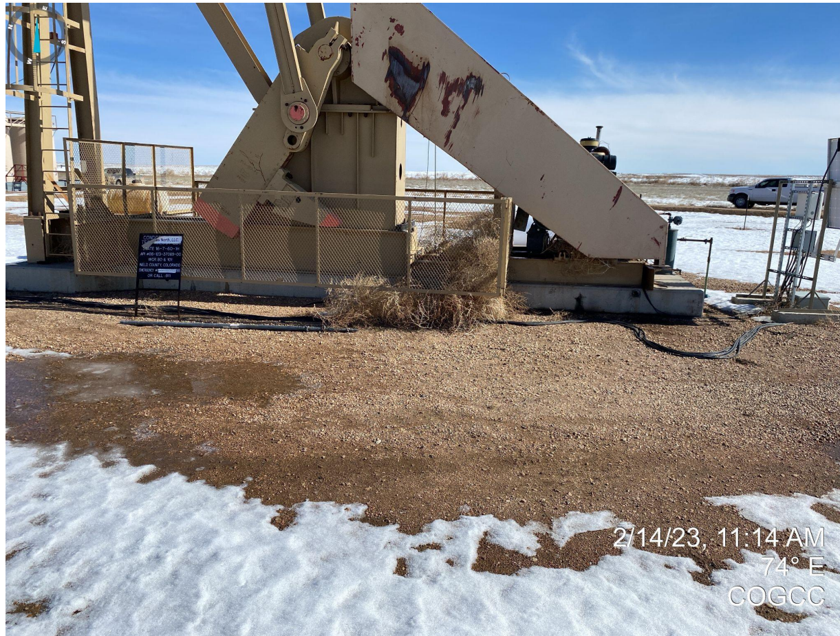
Photo 7. Facing east at pump jack; tumbleweed accumulations within equipment are considered debris and need to be removed as they are a potential fire hazard.
