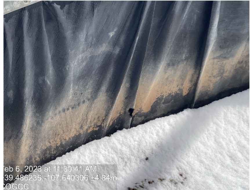
Holes in containment
