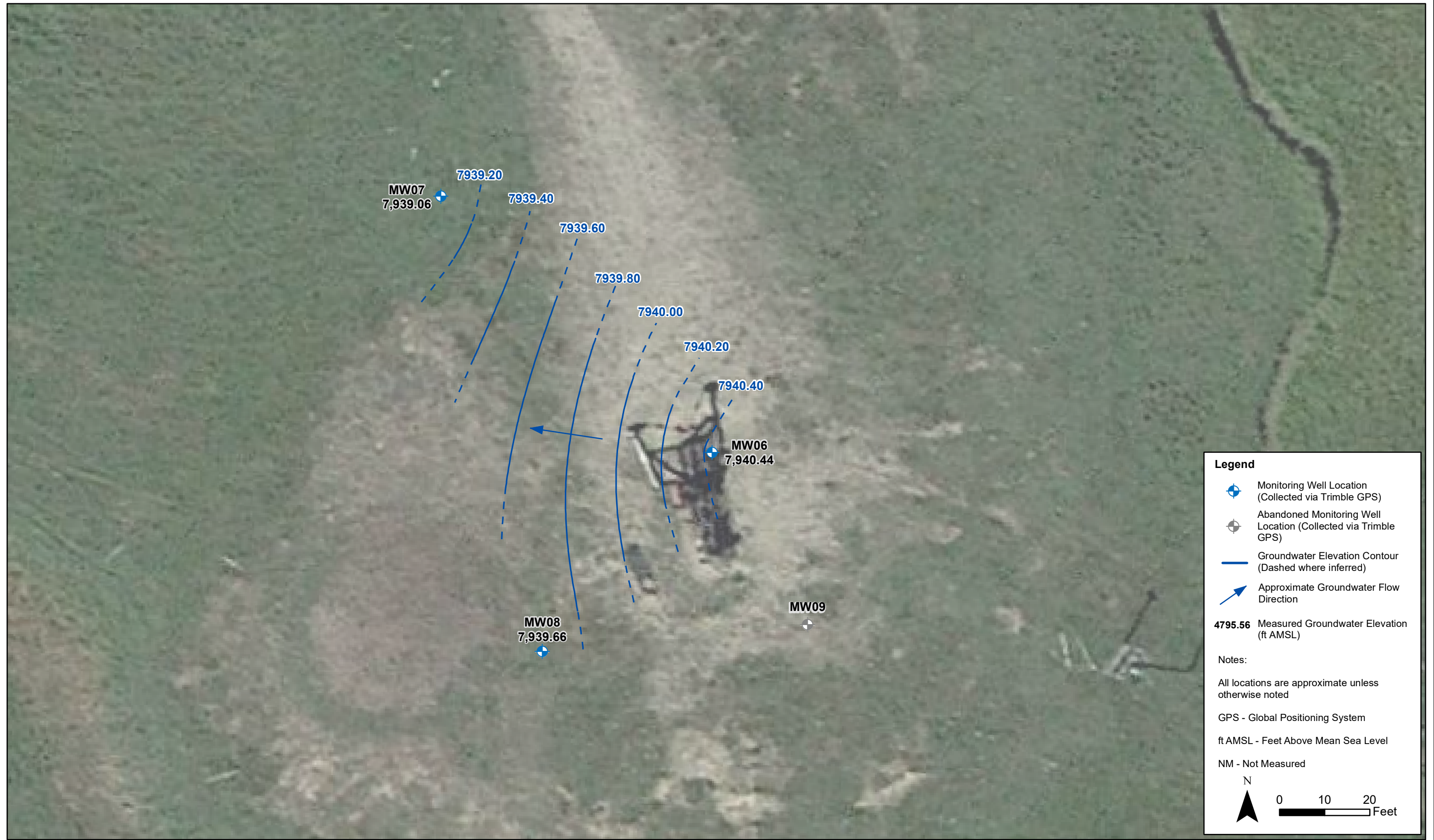
Groundwater Elevation Contour Map (November 9, 2022)
