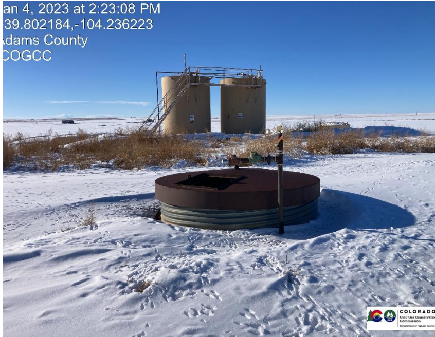
Pic 3 pit with steel pipe inside, needs cover
