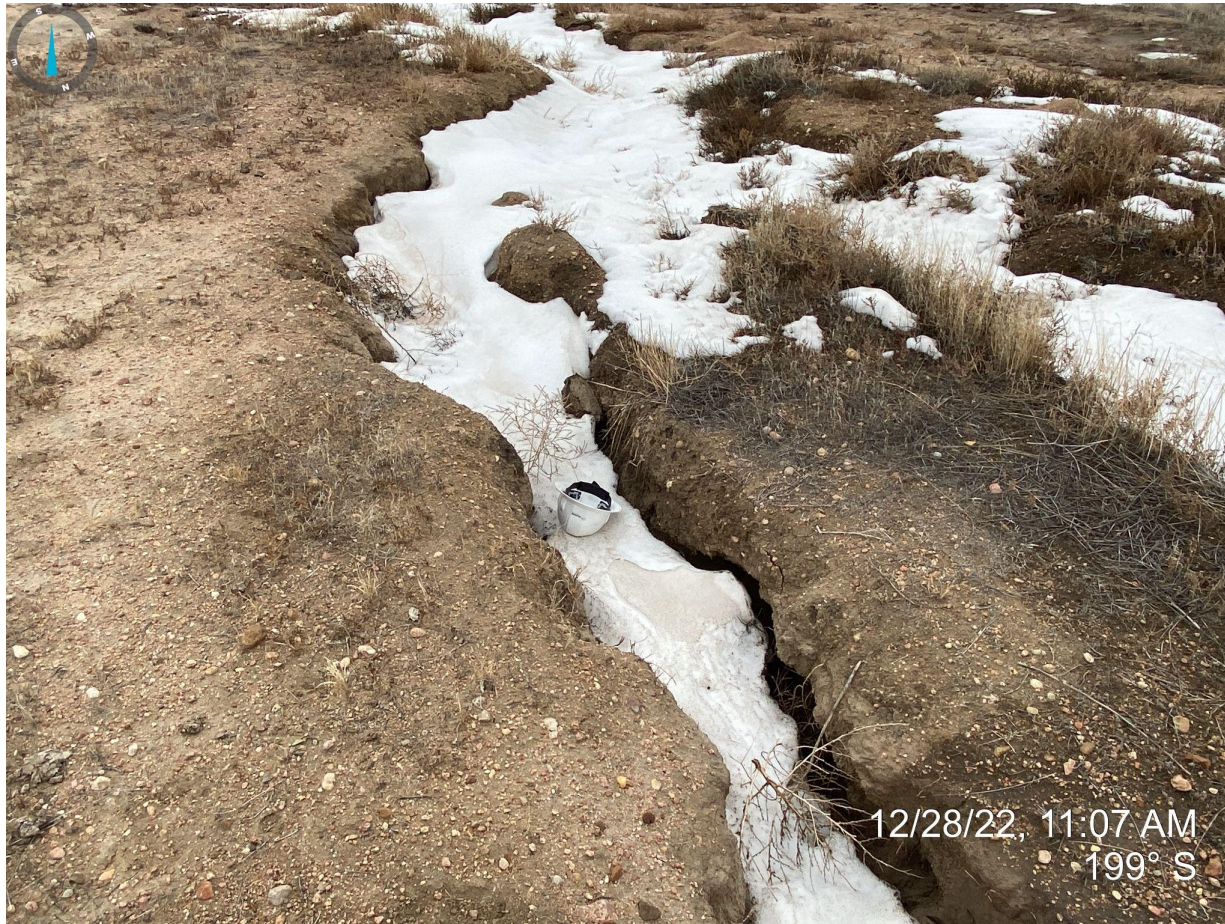
Photo 8. Taken approximately 175' from the access road, facing south. Gully was approximately 10" deep to top of snow cover, possibly deeper under the snow; hard hat for scale.
