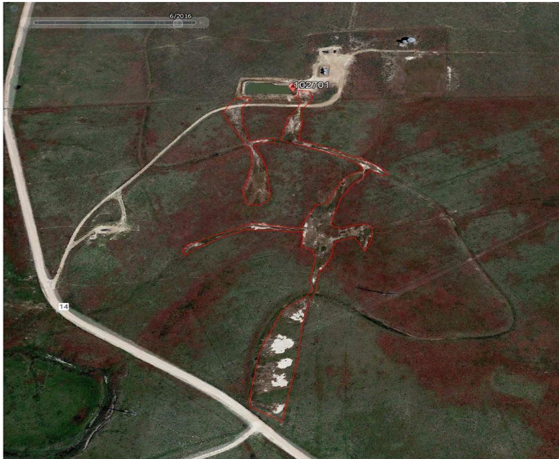
Photo 24. Google Earth aerial imagery taken circa 2016 illustrating the extent (outlined in red) of the salt kill impacted area. The Operator shall delineate the horizontal and vertical extent of the salt kill area and provide that information in a Supplemental Form 27.
