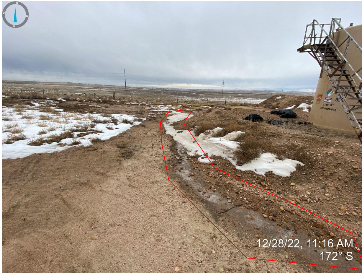
Photo 17. Facing south near the produced water tank. Picture shows evidence of rill/gully erosion occurring on the location with no apparent stormwater BMPs being implemented.
