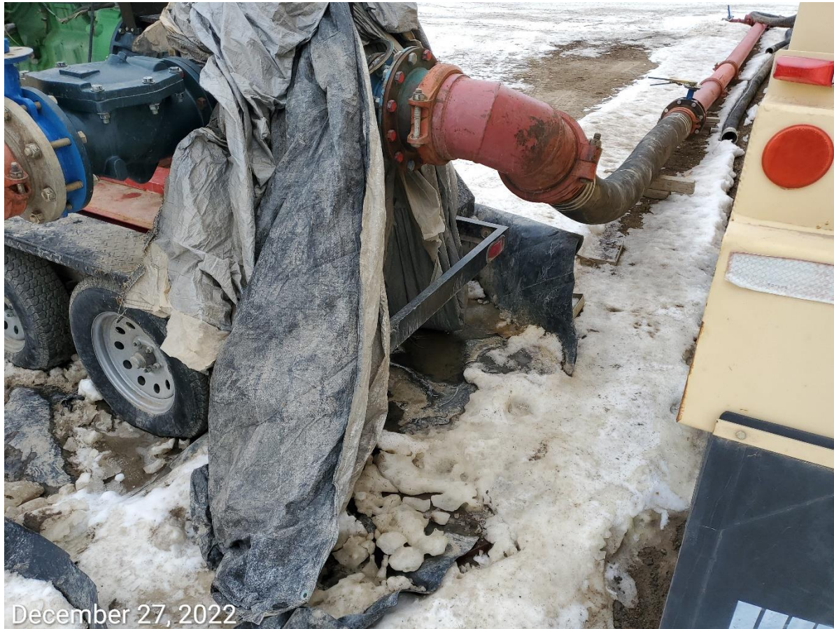
Photo 6: Photo taken from the pump observed on the east end of the Location. Photo shows secondary containment at pump is not in proper functioning condition/inadequate to contain a spill or release
