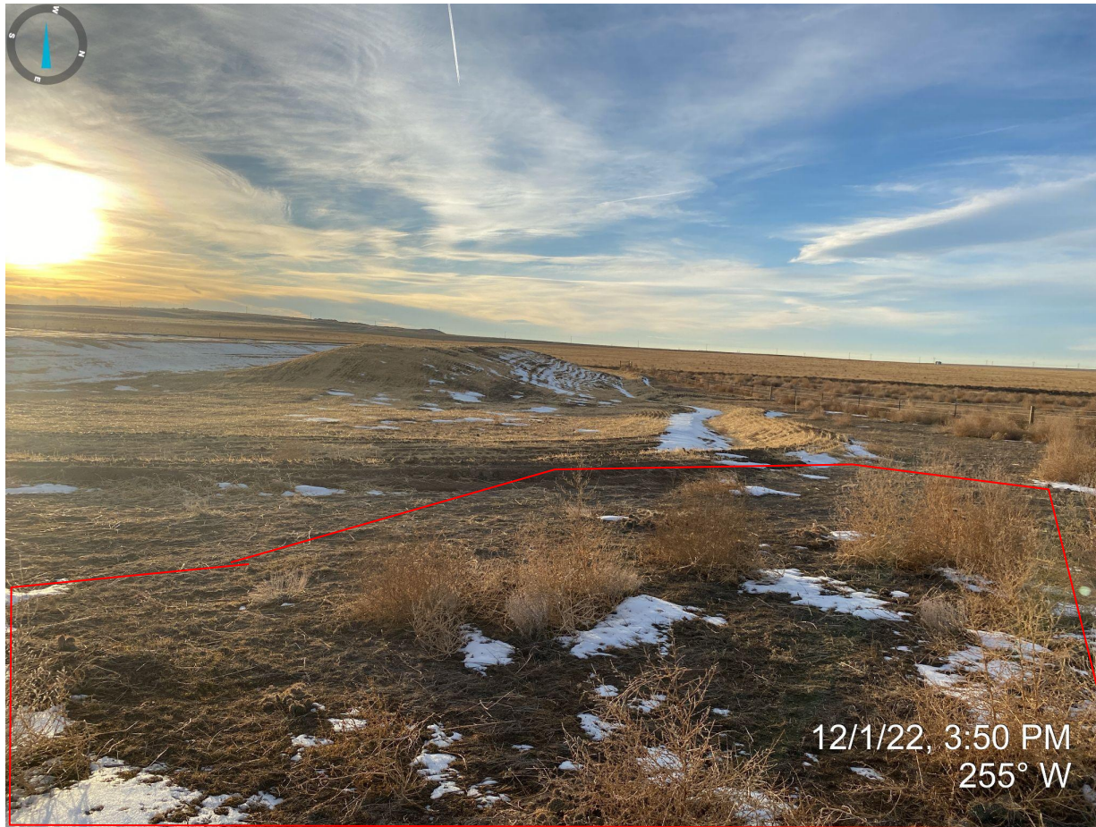
Photo 8. Facing west from the northeast corner of location. Photo illustrates perimeter ditch and berm and topsoil stockpile in background. Undesirable vegetation (e.g. kochia and russian thistle) observed; this is considered debris and needs to be managed/removed.
