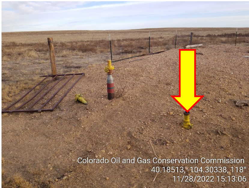
Photo 1 – TA Wellhead – Unmarked Flowline Riser
