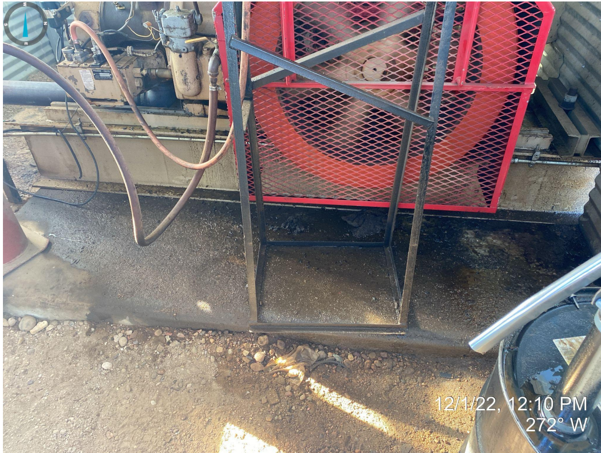
Photo 3. Close-up photo of pump jack motor, illustrating the oily stained/saturated foundation.
