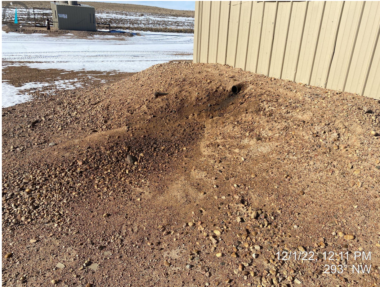
Photo 5. Taken from the southern end of pump jack, facing northwest. Photo illustrates oily stained soil near exhaust.
