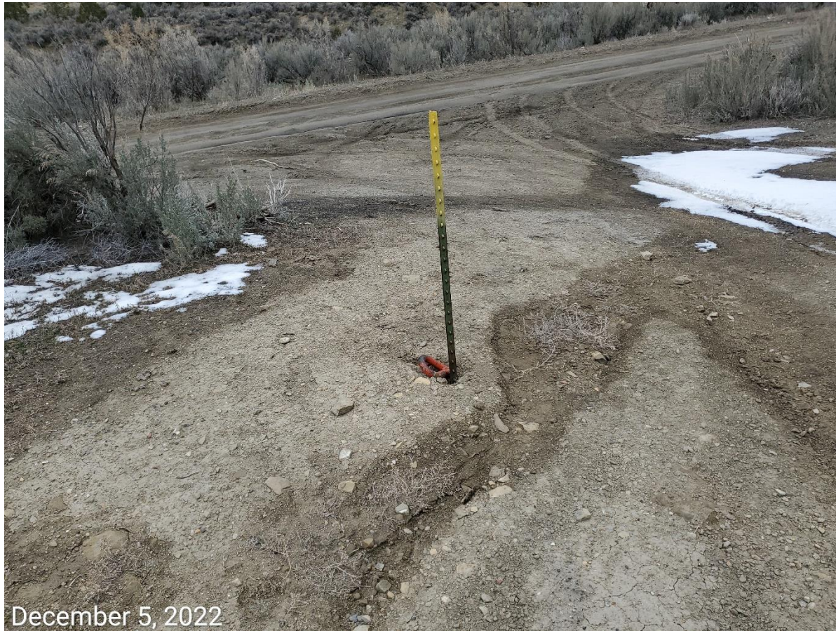
Photo 3: Photo example showing anchors with required marking.
