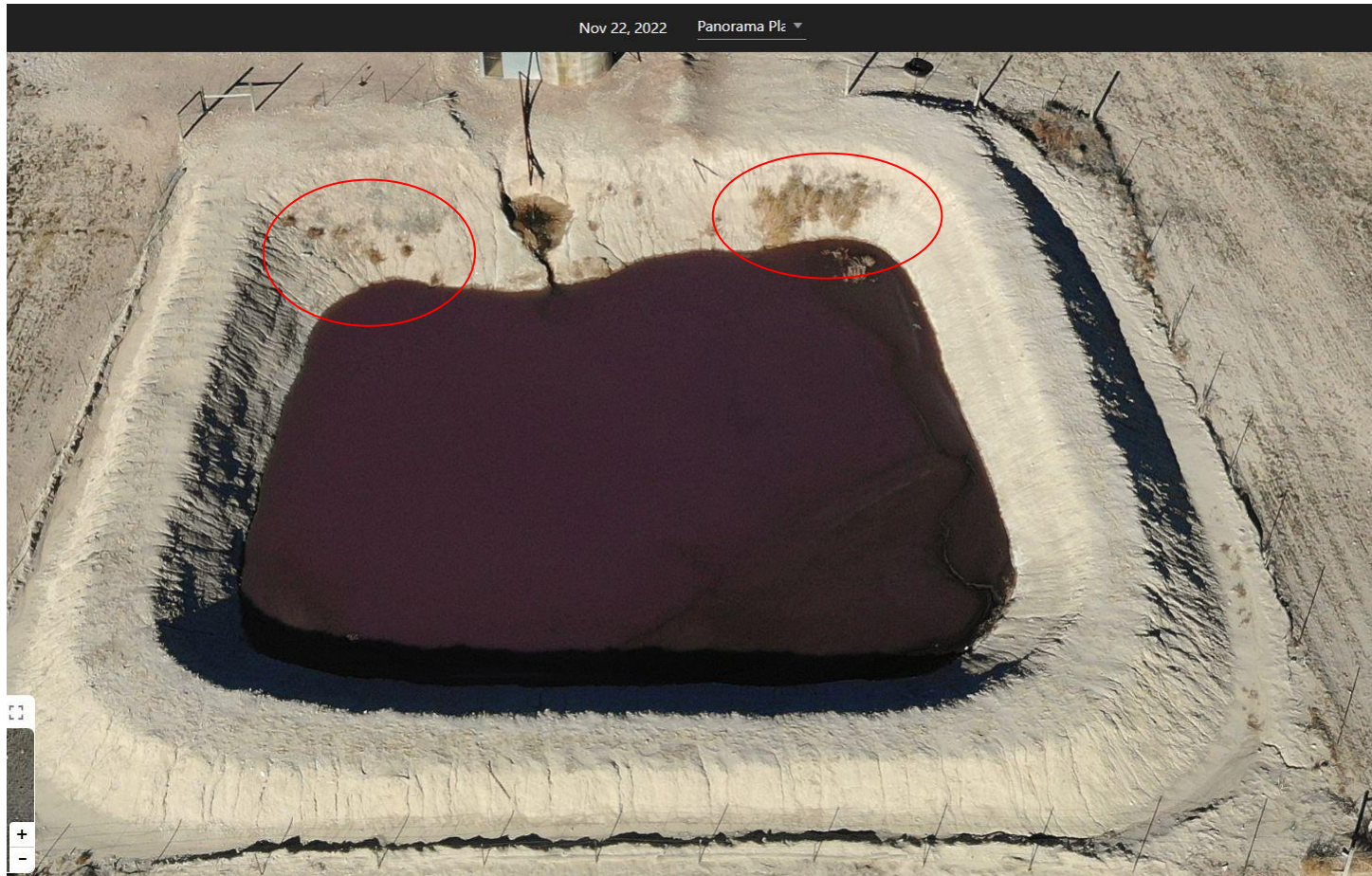
Photo 8. Drone aerial imagery taken from the southern part of the location, facing north. Photo illustrates the presence of rill and gully erosion that is occurring on all pit walls from stormwater run-on and run-off. Also observed is undesirable vegetation (e.g. kochia) in red and the oil skim on the surface of the water.
