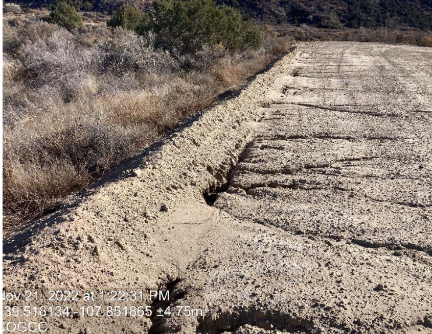
Erosion, tunneling through berm and sediment migration
