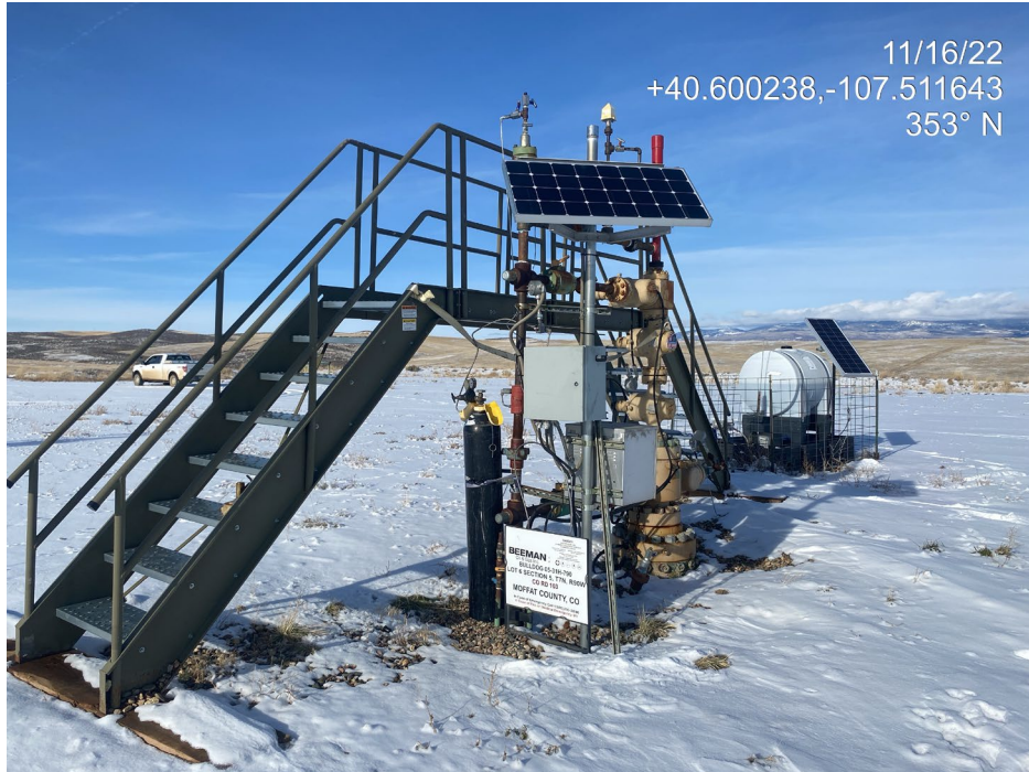
Photo 2. Photo shows the well sign lacks the well API number. See below for close-up.
