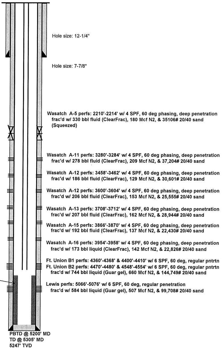
CO with undergauge bit to 5,186', scraper held up at 4,688', CO w/ 3.85" watermelon mill to 4,745'
