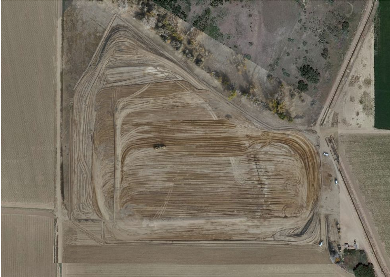
Photo 1. Drone aerial imagery illustrates the Garnet/21-K Pad with an approximate disturbance area of 12.95 acres. There are two topsoil stockpiles located along the north and southeastern location.
