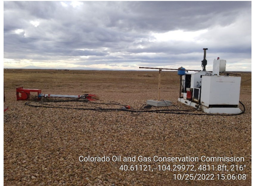
Photo 2 – Unused Hydraulic Pumping Unit and Engine
