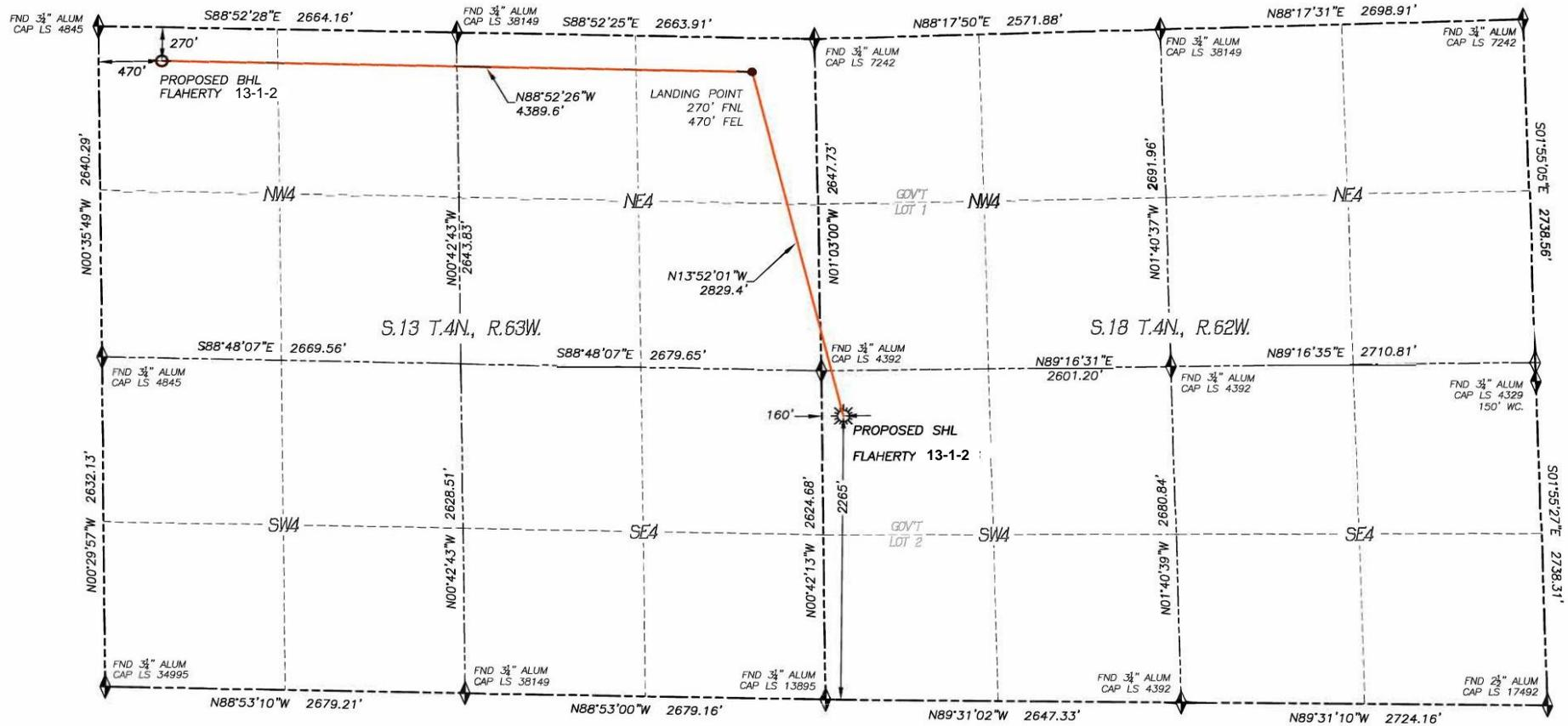
IN ACCORDANCE WITH A REQUEST FROM CONFLUENCE RESOURCES, DALEY LAND SURVEYING, INC. HAS DETERMINED THE SURFACE LOCATION OF THE FLAHERTY 13-1-2 WELL TO BE 2265' FSL, 160' FWL, AS MEASURED AT NINETY (90) DEGREES FROM THE SECTION LINES OF SECTION 18, TOWNSHIP 4 NORTH, RANGE 62 WEST AND THE BOTTOM HOLE LOCATION TO BE 270' FNL, 470' FWL, AS MEASURED AT NINETY (90) DEGREES FROM THE SECTION LINES OF SECTION 13, TOWNSHIP 4 NORTH, RANGE 63 WEST, OF THE 6TH PRINCIPAL MERIDIAN, WELD COUNTY, COLORADO.
