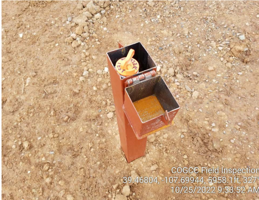
Photo #6 – Monitoring well in Remediation Project area.
