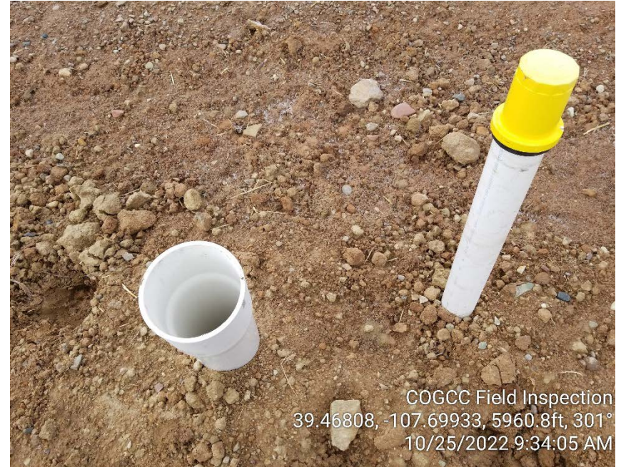
Photo #7 – PVC risers in Remediation Project area.
