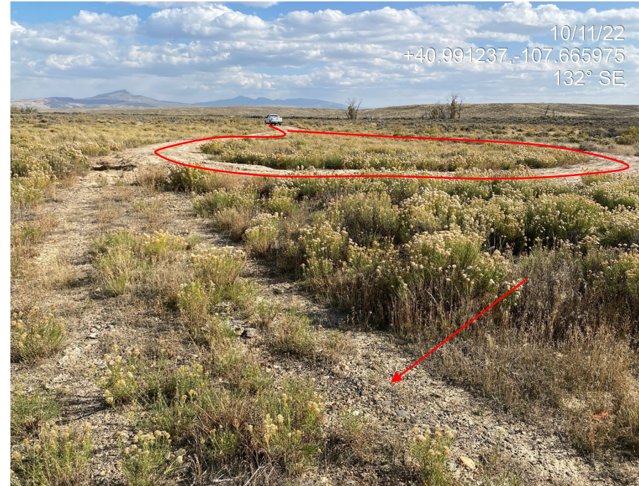
Photo 4. Photo taken to the west shows the access road remains. Soils has been spread over the top. Also pictured in the foreground is an unreclaimed access road to another Location operated by Mull Drilling Company to the west. The portion of access road pictured is on Location 313080. Soils are compacted and gravel remains.
