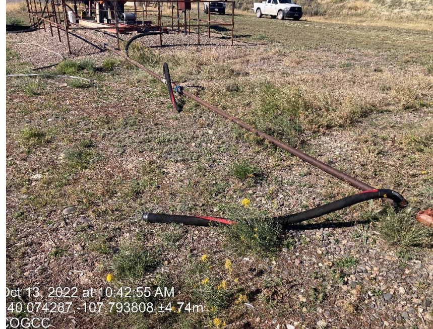
Stored equipment lines are open ended
