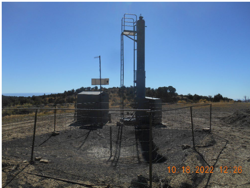
Meter housing, Dehydrator and blowdown pit with fence
