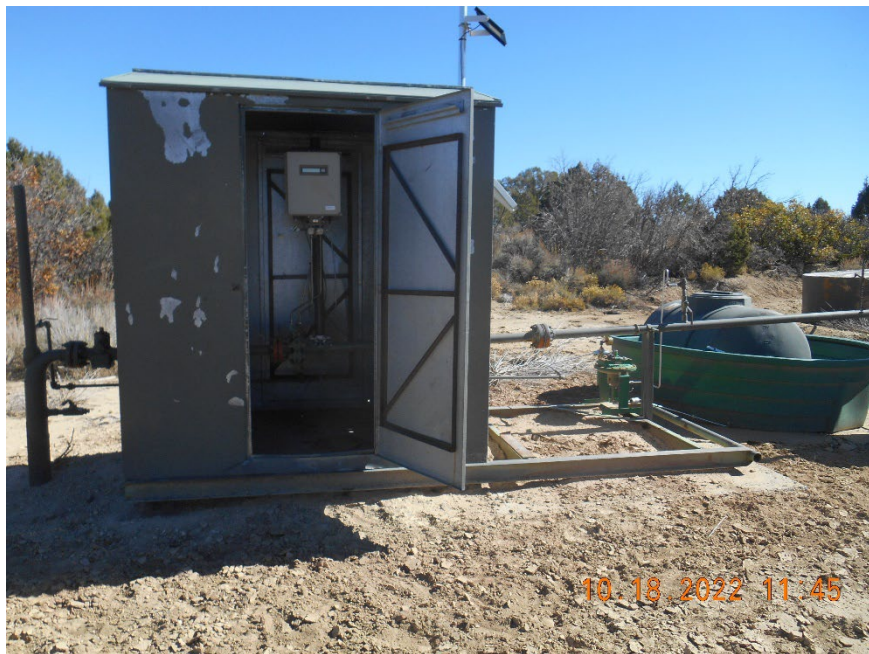
Meter housing with Secondary containment of chemicals
