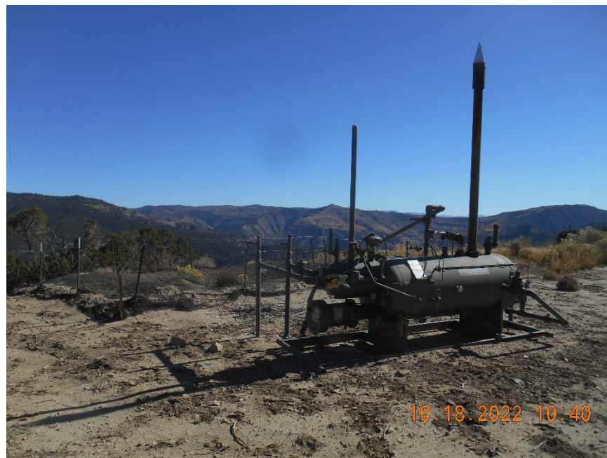
Separator. Blowdown pit with fence and netting.
