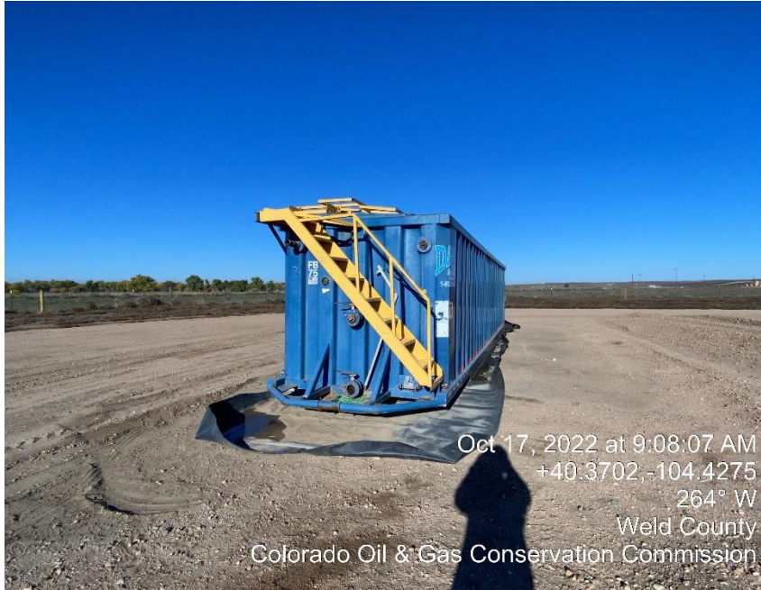
Photo #1 Inadequate Berm/ Unused Frac Tank
