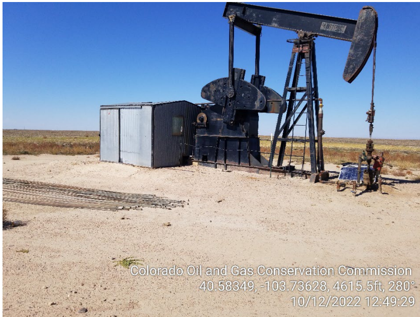
Photo 5 – Pumping Unit – Unused Rods
