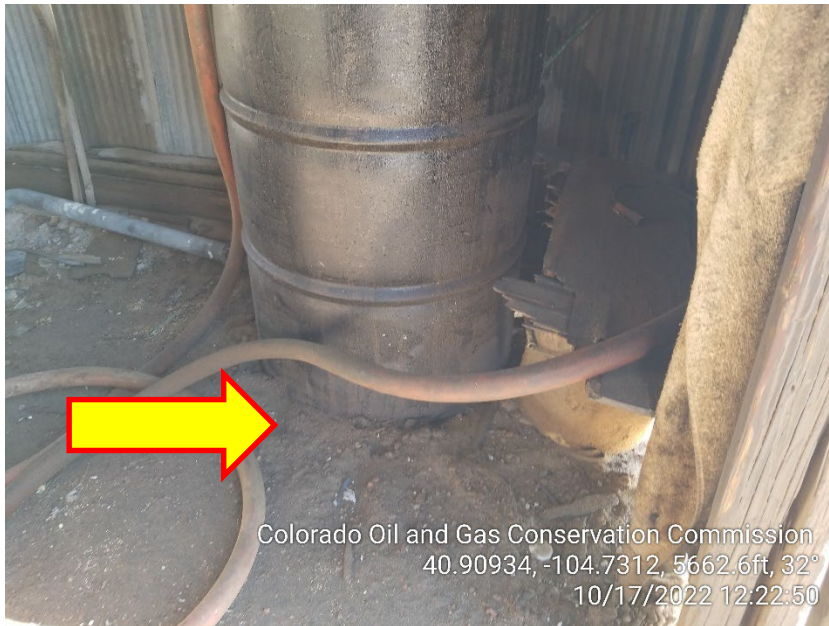
Photo 7 – Inside Gas Engine House – Stained Soil
