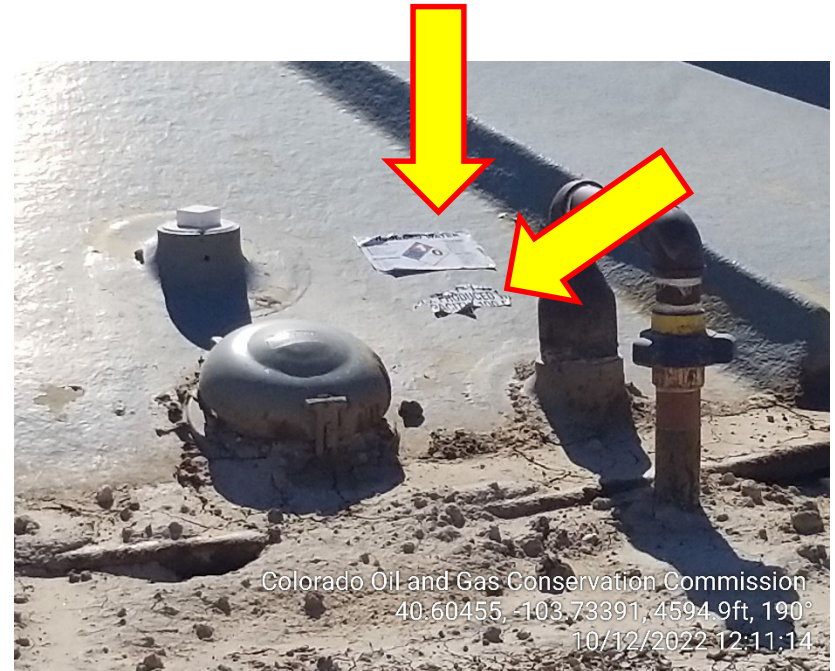
Photo 6 – Labels have faded, no longer Visible
