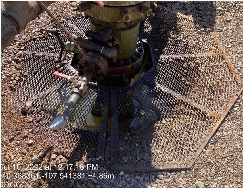
Cellar full of fluid possible hydrocarbons
