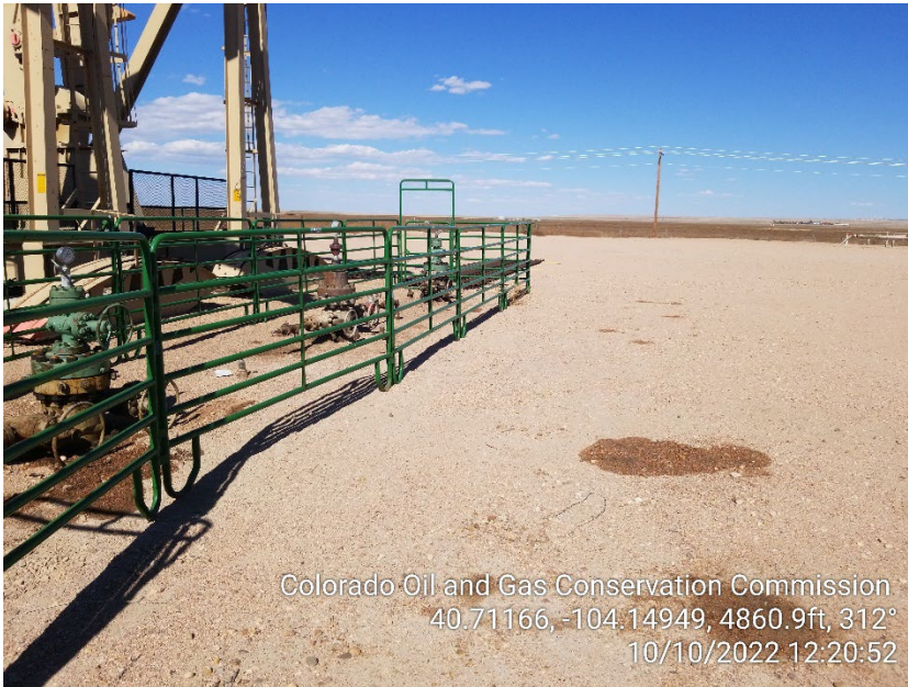
Photo 1 – Stained Soil at Wellheads
