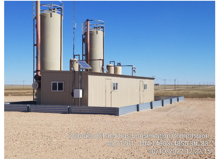
Photo 2 – North Heater Treaters
