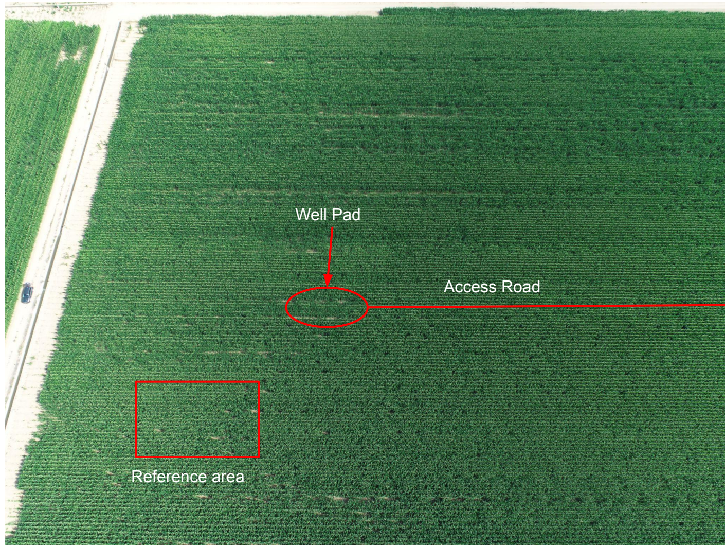
Photo 2. Overview photo of the well pad and access road taken from the southern edge facing north using a drone. Note: well pad and access road appear consistent with the adjacent crop reference area.
