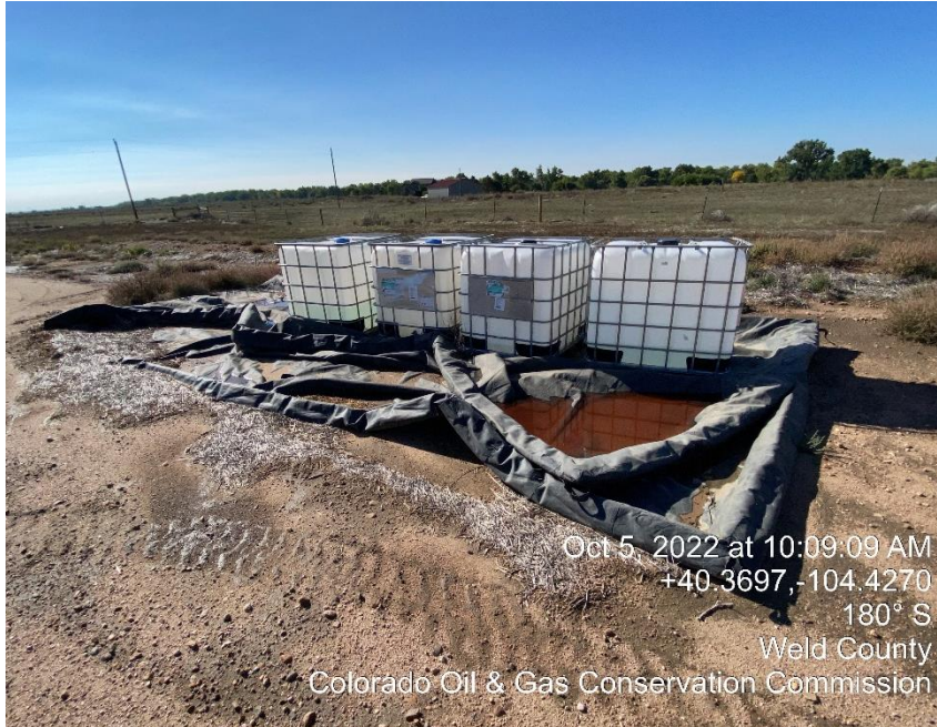
Photo #5 Inadequate Berms/ Unused chemical totes
