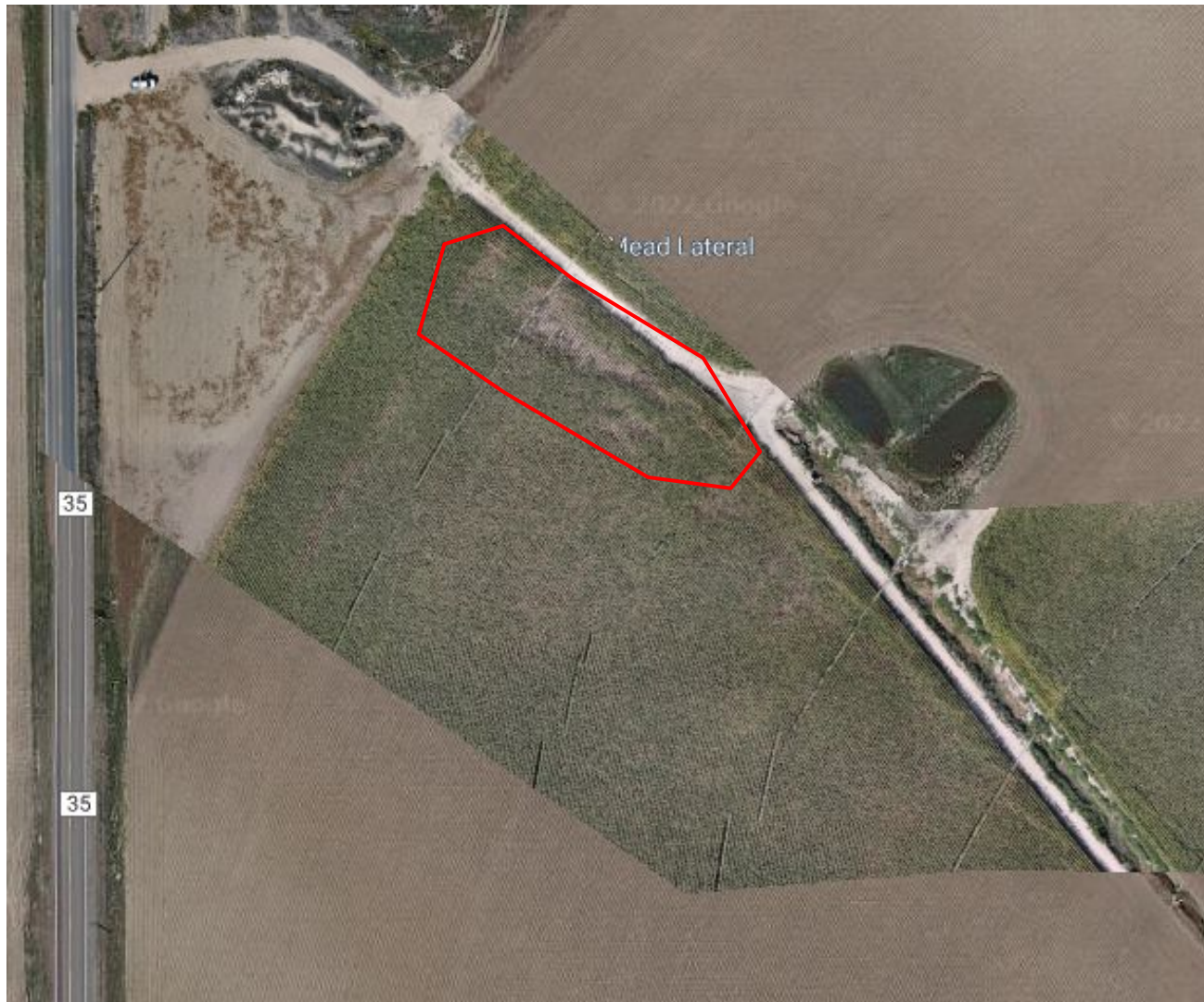
Photo 3. COGCC drone orthomosaic imagery illustrates an ~200' flowline length where crop growth is not reflective of reference areas.
