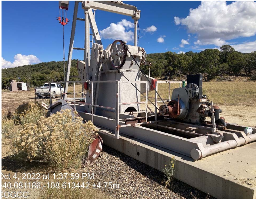
Guard missing from pump jack
