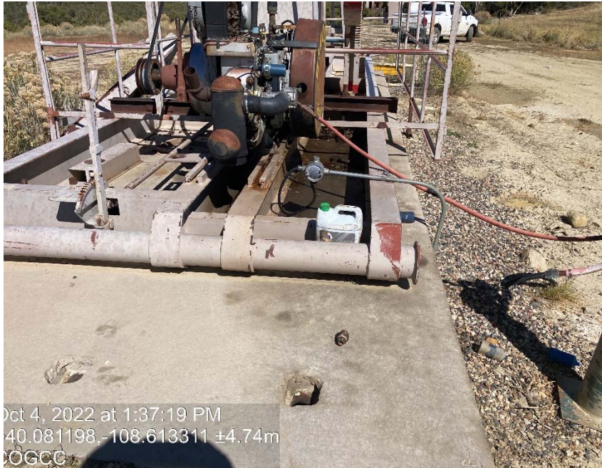
Staining and bottle not contained
