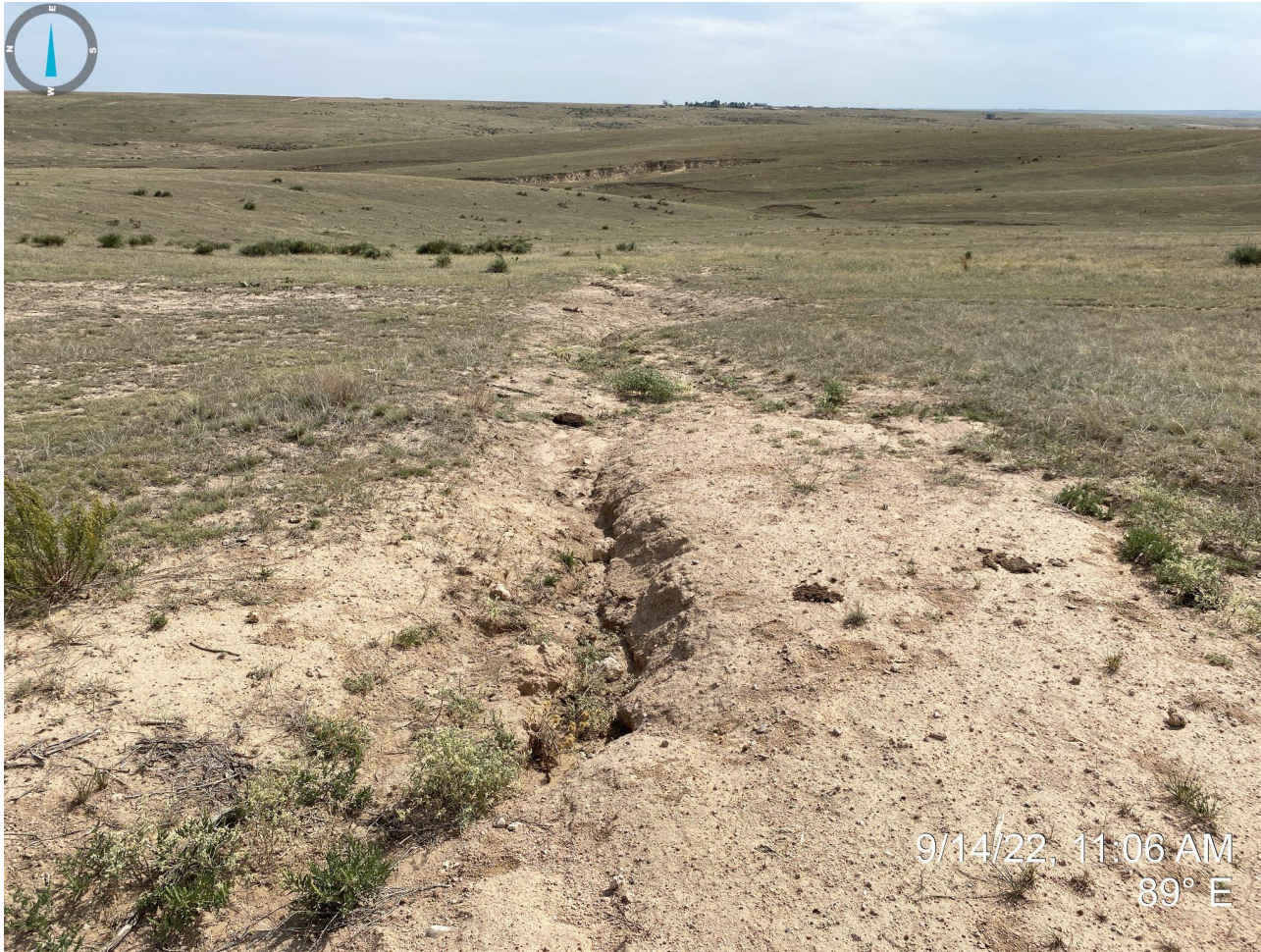
Photo 3. Taken from eastern portion of location, facing east. Photo illustrates gully erosion approximately 1.5' deep x 115' length x 10' wide. Extent of erosion is leaving permitted location and contributing to offsite sediment deposition; no erosion control BMPs observed during inspection.
