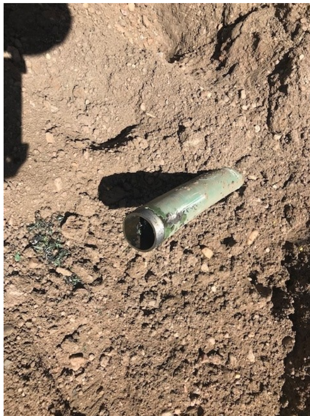
#10 – Former Flowline at Separator Just Before Filling with Cement
