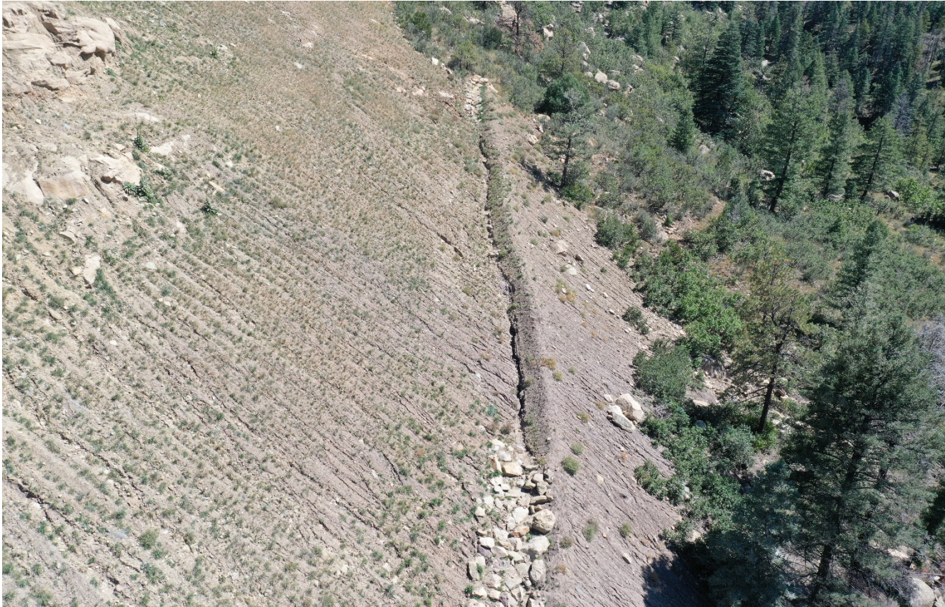
Photo 4. Facing east down at the location. A large berm was installed at the bottom of the location. The area to the right of the berm does not appear to have vegetation establish and may need to be hand seeded this fall.
