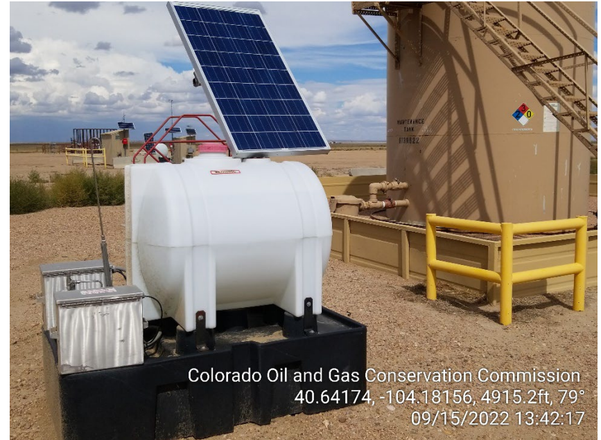
Photo 18 – Unused Methonal Maintenance Tank
