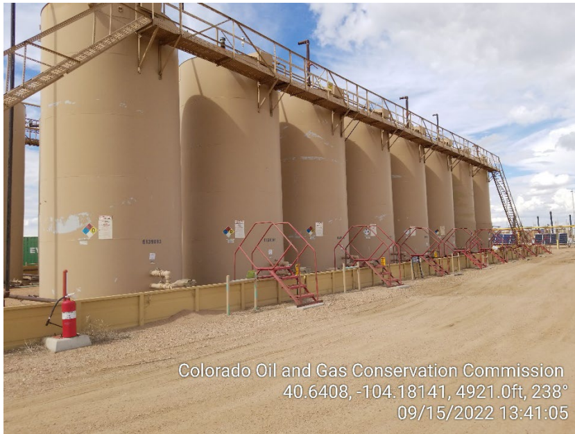
Photo 15 – Tank Battery
