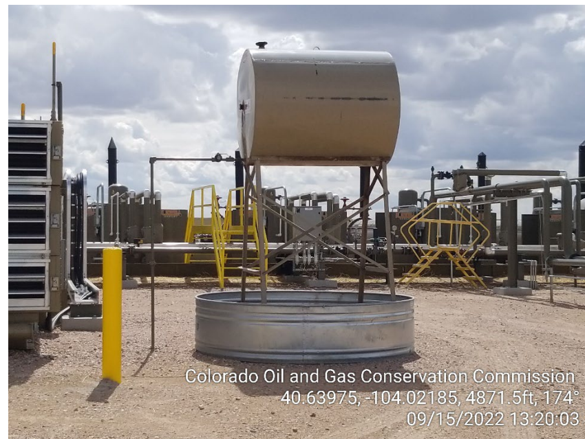
Photo 18 – Wildlife Netting missing on Day Tank
