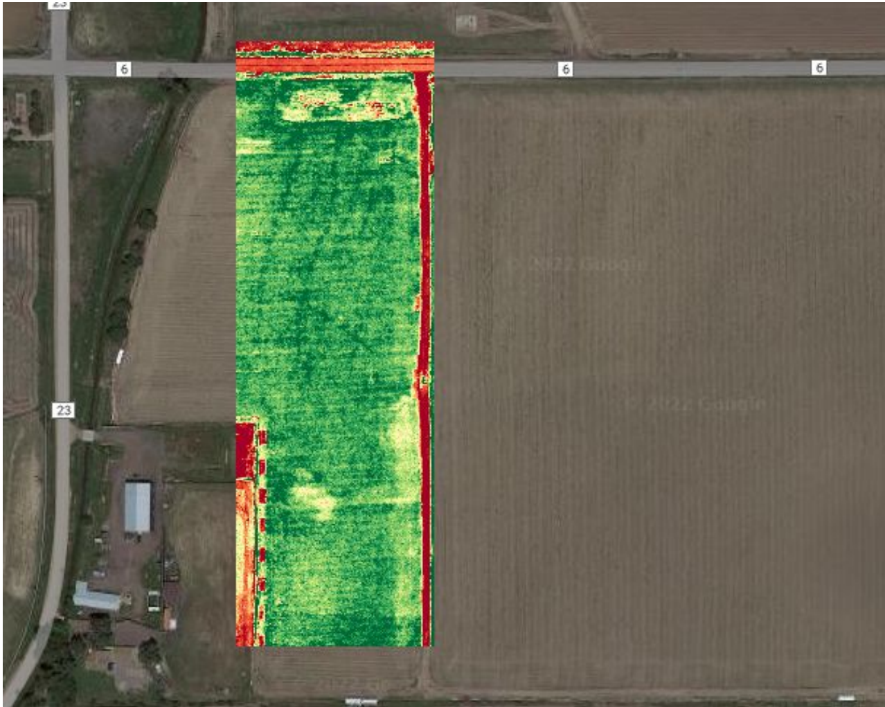
Photo 7. COGCC drone imagery illustrates the Visible Atmospherically Resistant Index which measures how green an image is. Based on this image, there is no observed issues along the flowline area. Note- the tank battery has red coloration which indicates bare soil.
