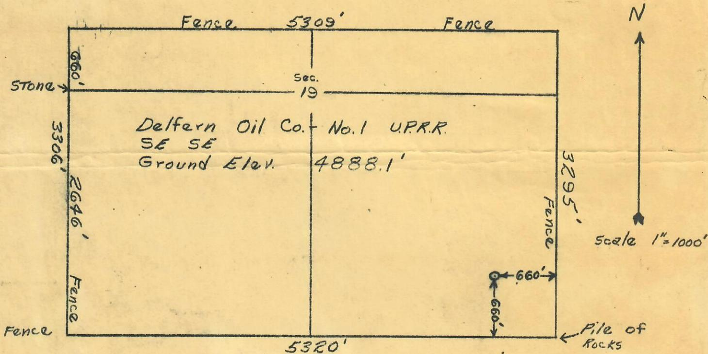
I hereby certify that the above plat is an accurate representation of a correct survey showing the location of Delphern Oil Co. U.P.R.R. No. 1 Oilwell in SE $\frac{1}{4}$ SE $\frac{1}{4}$  Sec. 19 T12N R55W 6PM. Logan County, Colorado. The elevation of the ground at the well is 4888.1 feet above sea level from U.S.C. & G.S. B.M.
